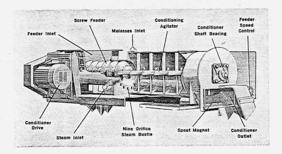
$18 \times 56$  Dual Drive Feeder-Conditioner, with independently driven constant speed agitator and variable speed feed screw.
